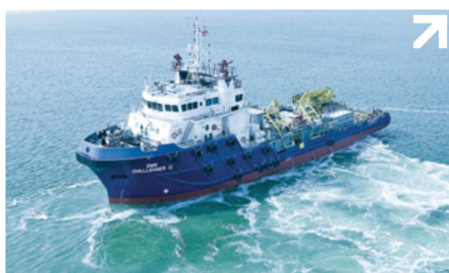
DMS Challenger II is a 58m, 4000bhp Multi-Purpose Support Vessel operating in the Arabian Gulf.
